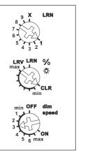
If the upper rotary switch is set to X, special functions are active, which must be settled with the PC Tool PCT14. The minimum brightness (fully dimmed) is adjustable with the % **Ö** rotary switch. The dimming speed is adjustable using the
